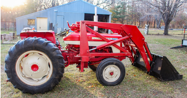
International 444 Gas Tractor Wide Front, 3 Point, Live Hydraulic, Diff. Lock, 8 Speed High/Low Transmission, Power Steering, 14.9-28 Rubber, Hydraulic Loader with Float, Ser. #07588
