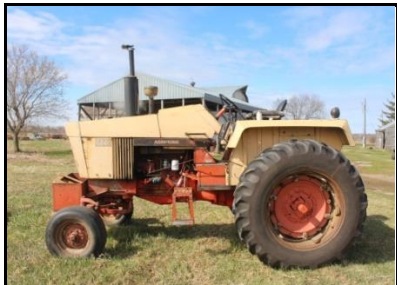
Case Agri King 870 Diesel Tractor, Wide Front, 3 Point, Dual Hyd., Power Shift, 18.4 x 34 Rubber
