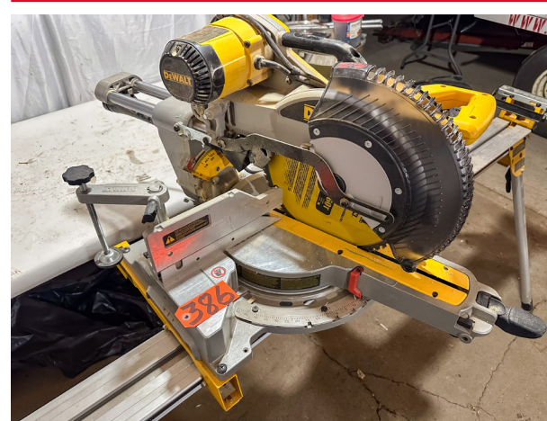
DeWalt DWS780 12" Double Bevel Sliding Compound Miter Saw on DeWalt Sliding Stand
