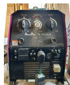
Thermal Arc AC/DC CC/CV Welding Generator Power-Plus TA 10/270H, 8500 KW, Honda Engine
