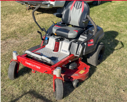
2020 Toro Timecutter Zero Turn Lawnmower MyRide Suspension System, 42" Deck
