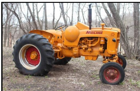
Minneapolis Moline 5 Star LP Gas Tractor, Wide Front
