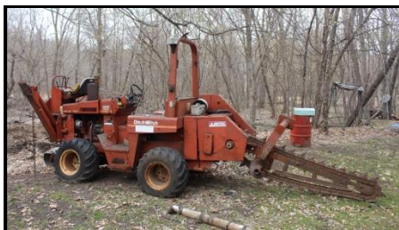
Ditch Witch 4010 Trencher, Deutz Diesel Engine With A420 Backhoe Attachment
